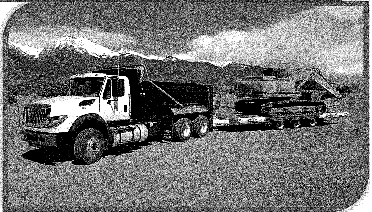
New International 7600 Dump Truck and Trail Max 60K lbs capacity trailer carrying 45K lb 9030 Case Excavator
