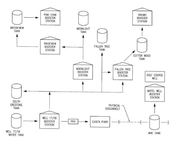
Figure 4: Distribution System Process Flow Diagram
