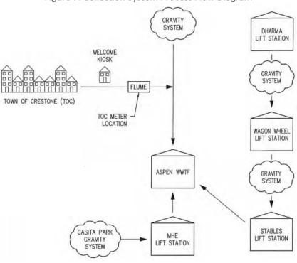
Figure 7: Collection System Process Flow Diagram
