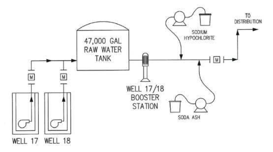
Figure 3: Raw Water Supply and Treatment Process Flow Diagram
