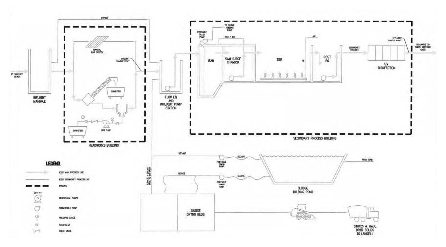
Figure 8: Wastewater Treatment Plant Process Flow Diagram
