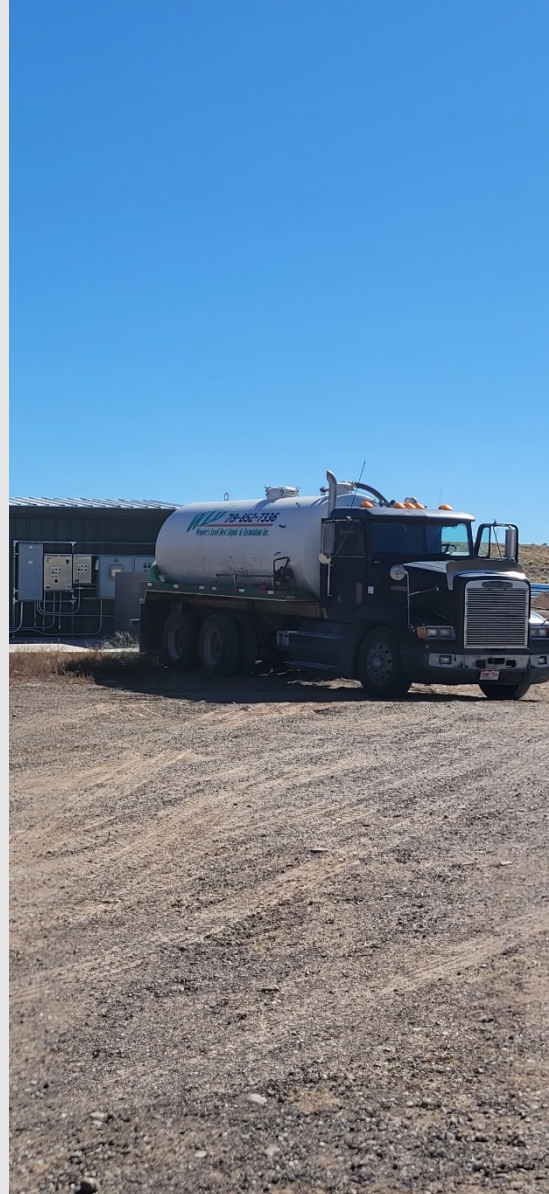
Picture of extra pump truck hauling Wastewater and dumping at Aspen Waste Water Treatment Plant
